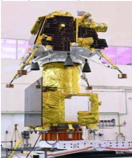
Chandrayaan-3 Integrated Module in clean room
